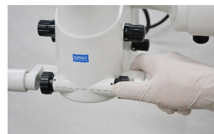
Adjust the fine focus knob
